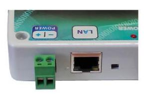
the + terminal on the module. Connect negative terminal of the power supply to - terminal of the module.
