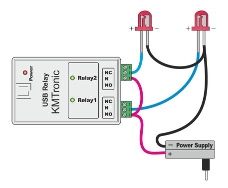
Above images shows basic connection diagram that can be used in most of the situations. The connection diagram is same for both AC and DC loads. Please make sure to use a freewheeling diode or snubber circuit if the load is inductive. More details about using inductive loads are available
